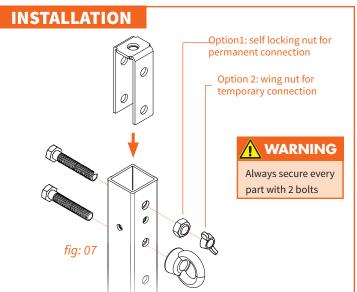
In case of assembling a "Single rigger" connect two Nutplate sets, at the top and bottom of the profile. When assembling a "Down rigger", connect the Nut plate set at the top of the profiles.
