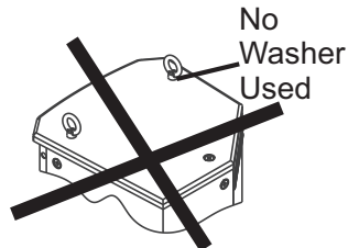
Figure 4.8: Eyebolt shown with and without washer
