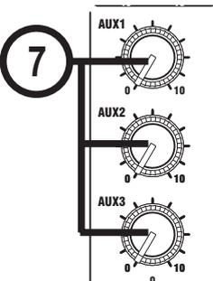
AUX SEND 1 is fixed pre-fade, AUX 2 is globally switchable between pre and post-fade (see master section on page 20). On the MPMi, Aux 3 is fixed post-fader.
