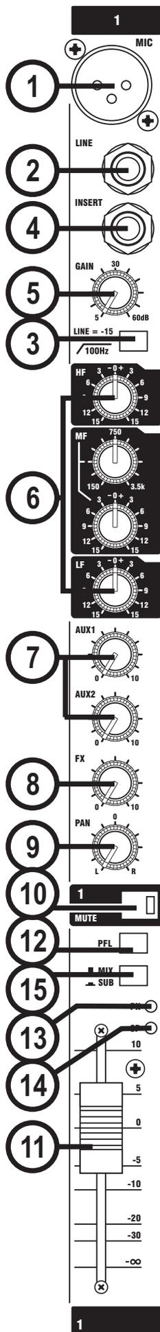
The Send may also be tapped off as an alternative pre-fade, pre-EQ direct output if required, using a lead with tip and ring shorted together so that the signal path is not interrupted (see below).
