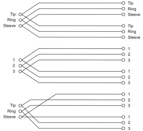
**Headphone Separator** Note: for every doubling of headphones the load impedance is halved. Do not go below 32 Ohms.
